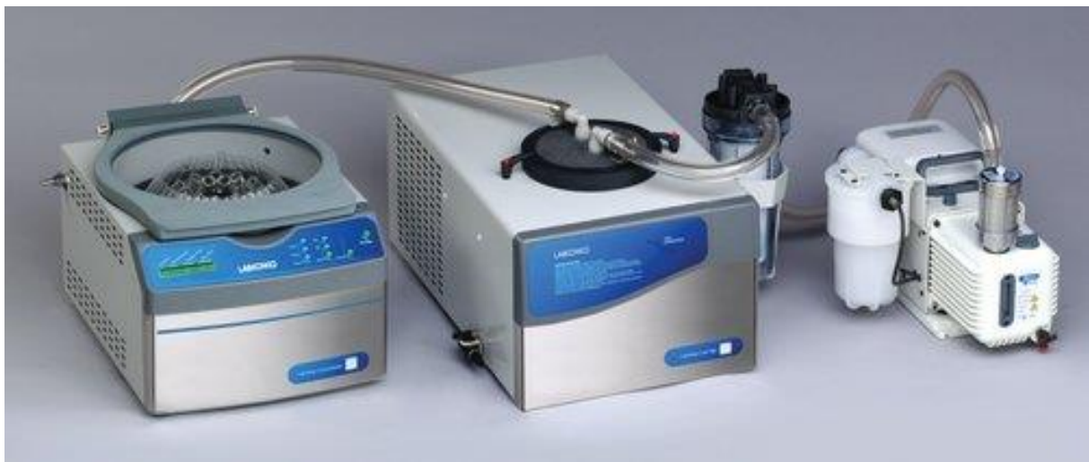
Figure 7. An example of centrifugal vacuum concentrator (left) equipped with a cold trap (middle) and driven by a vacuum pump (right).
